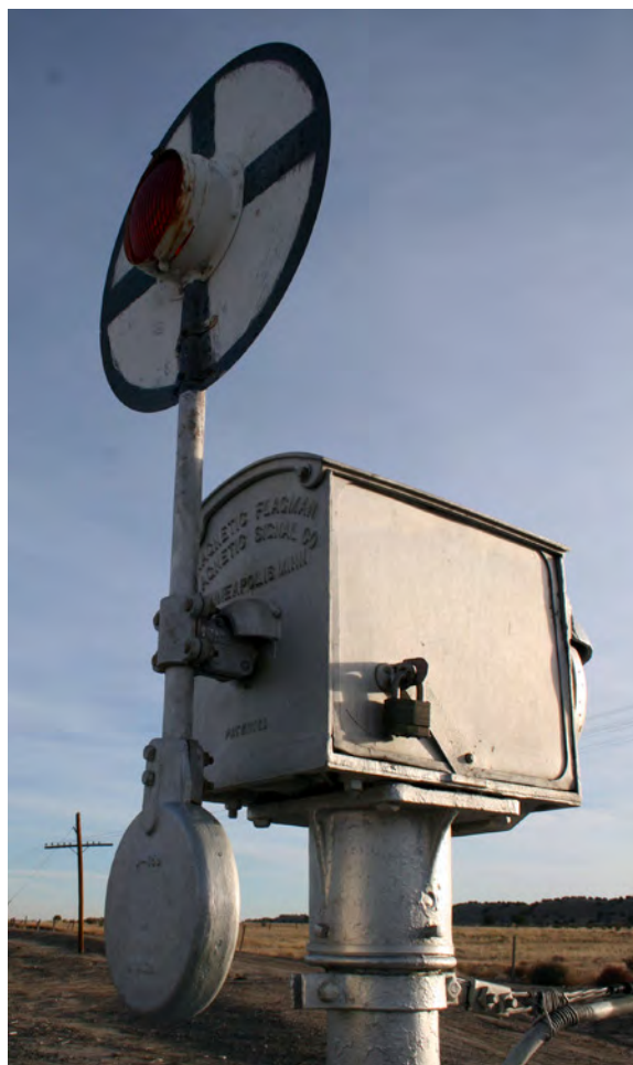
Above, the last active "Magnetic Flagman" on the Raton Pass line. Our travellers' timing was fortuitous: The old wigwag signal was replaced on March 9 of this year.
