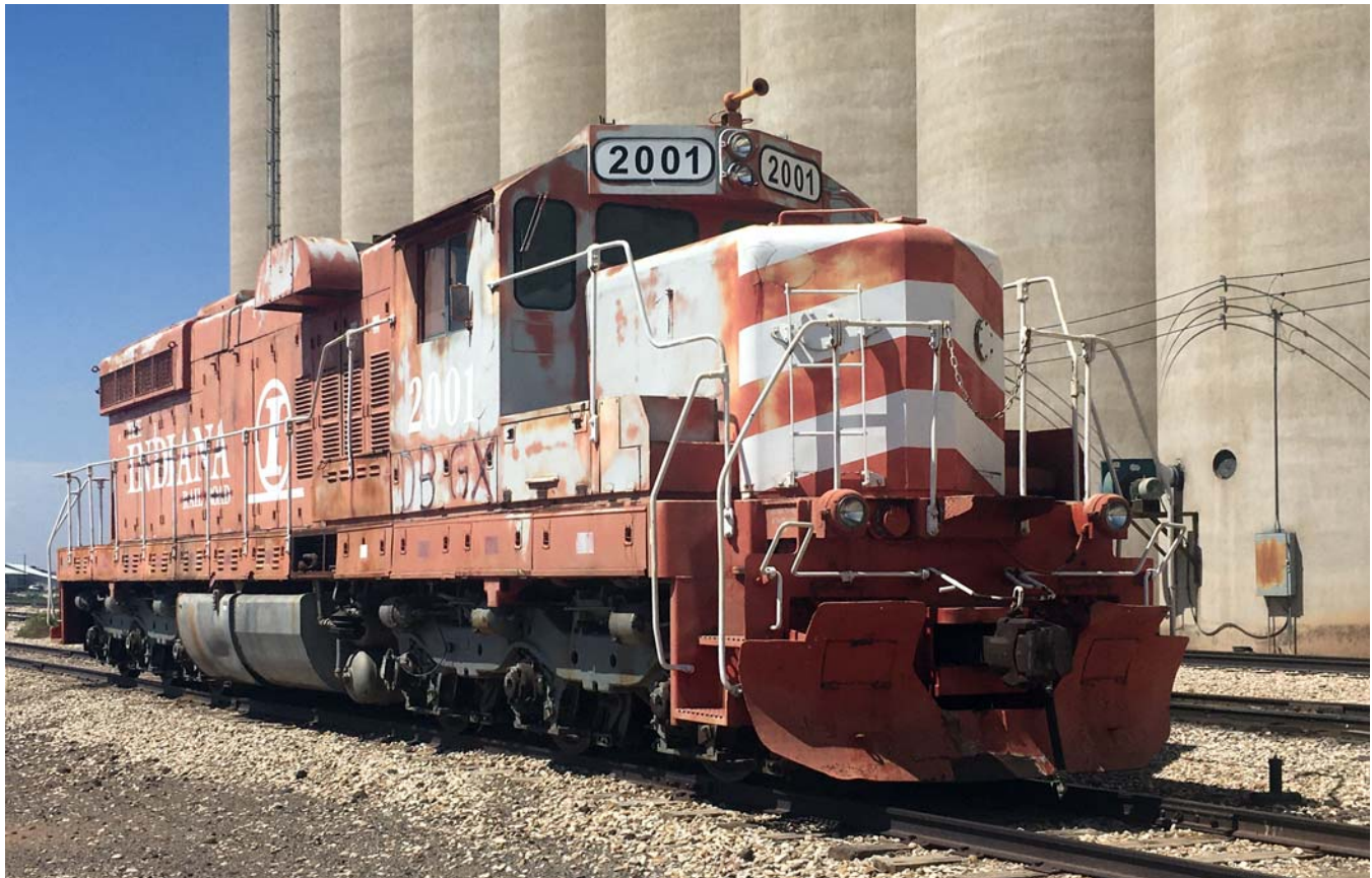
Above and right, Charles Goldmeyer came across this former Indiana Railroad EMD just north of Plainview. The locomotive was built as a high-nose SD7 in 1952 for Milwaukee Road. Since a rebuild, No. 2001 is now generally referred to as an SD10.
