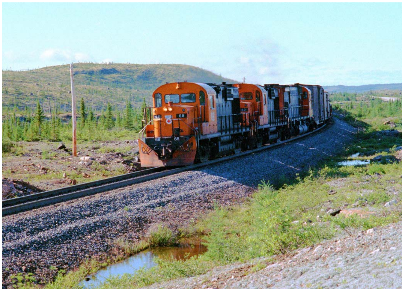
Above, a pair of MLW RS18s are teamed with an M636 on a Quebec Cartier Railway freight train. Leading is No. 68, built in 1960. The middle unit, No. 62, was built in 1959. The trailing M636's number is obscured.
