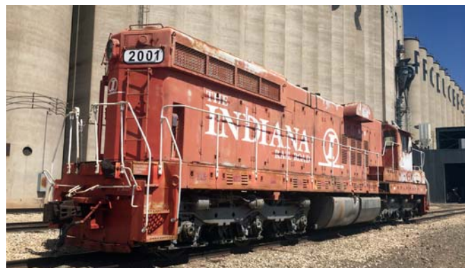
Above and right, Charles Goldmeyer came across this former Indiana Railroad EMD just north of Plainview. The locomotive was built as a high-nose SD7 in 1952 for Milwaukee Road. Since a rebuild, No. 2001 is now generally referred to as an SD10.
