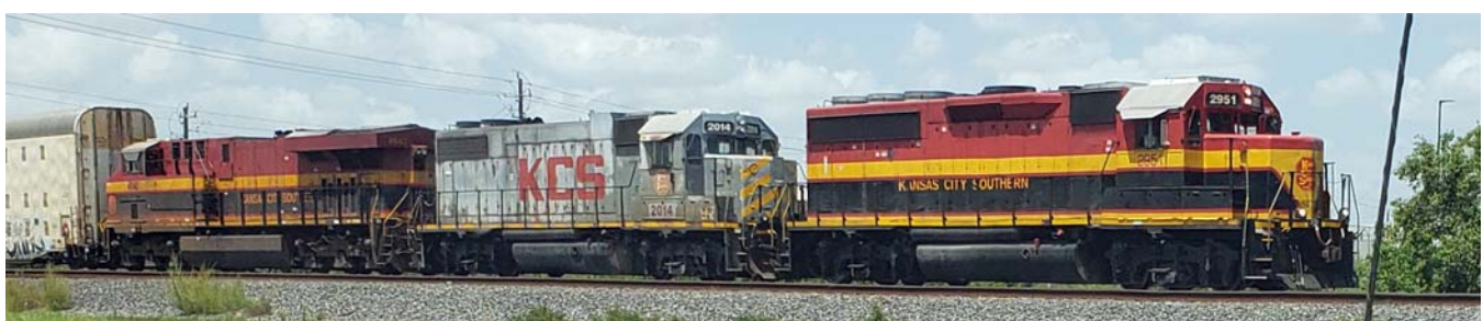
Below, Allan Melton caught this varied KCS lashup in Sugar Land. Leading the trio is No. 2951, a rebuilt EMD GP40-2 originally delivered to Frisco in 1979. Tattered gray No. 2014 is an EMD GP38-2 that started life in 1973 with Boston & Maine. The trailing unit, No. 4843, is a GE ES44C delivered to KCS in 2014.
