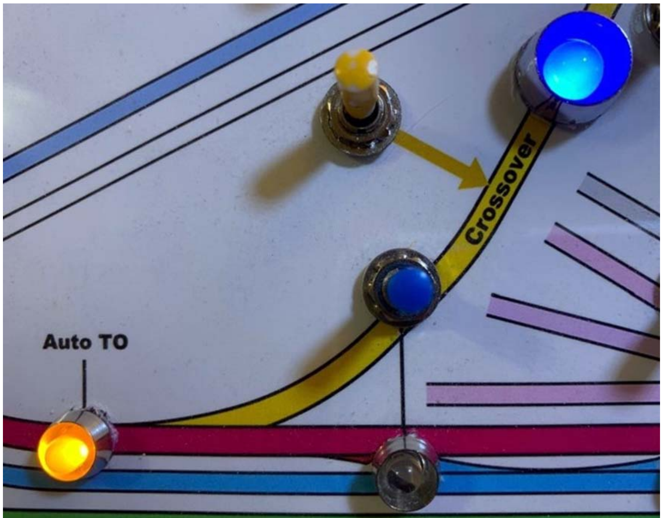
This photo shows a portion of my layout's remote panel, indicating a train is approaching the reverse loop turnout. The 8 mm blue LED confirms the presence of a train on the gold colored return track marked "Crossover". The 5 mm amber LED indicates the turnout has been automatically set to allow the train to proceed on the red colored track. The yellow and blue toggle switches and the unlit LED are not involved in the automatic turnout alignment function.
