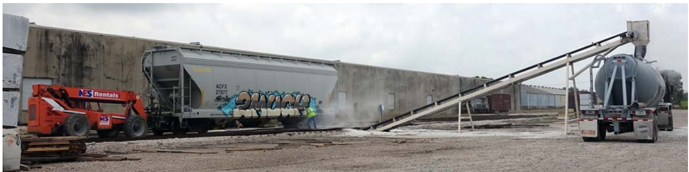
Hoppers carrying minerals were unloaded with this conveyor. The large forklift has been used to position the hopper bays over the drop pit. ACFX 27877 was the last revenue car unloaded at Genesis.
