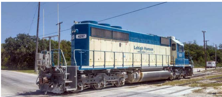
Lehigh Hanson SD40-2 No. 4297 working at Garden Ridge, Texas, earlier this year. The locomotive is now remote controlled, as evidenced by the equipment and antenna mounted on the rear of the locomotive. Photos by Leonard Ruback
