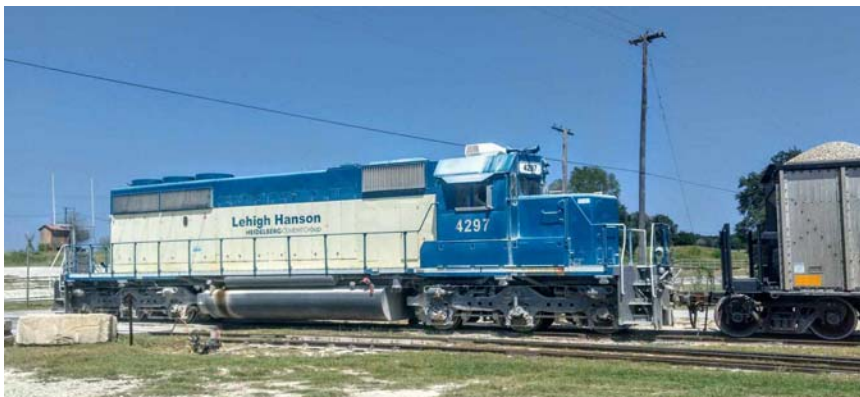
Lehigh Hanson SD40-2 No. 4297 working at Garden Ridge, Texas, earlier this year. The locomotive is now remote controlled, as evidenced by the equipment and antenna mounted on the rear of the locomotive. Photos by Leonard Ruback
