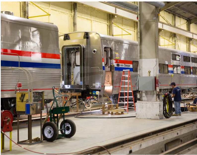
Above, the Viewliner II construction line. The new cars are being finished in a version of Amtrak's "Phase III" paint scheme that apparently will include new "Amtrak America" branding. Below, a Viewliner II car shell at the CAF USA shop in Elmira, N.Y. Photos this page courtesy of Amtrak.
