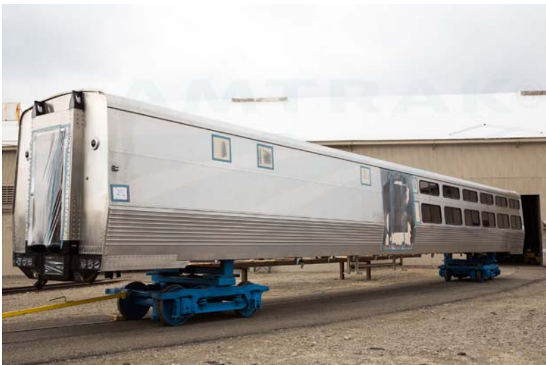
Above, the Viewliner II construction line. The new cars are being finished in a version of Amtrak's "Phase III" paint scheme that apparently will include new "Amtrak America" branding. Below, a Viewliner II car shell at the CAF USA shop in Elmira, N.Y. Photos this page courtesy of Amtrak.
