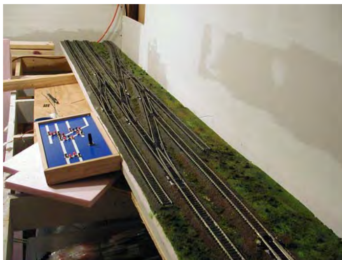
Above, the track plan takes shape. Two below, control panel and scenery: The roadbed was carved into the foam base. Photos by Steve Lancaster
