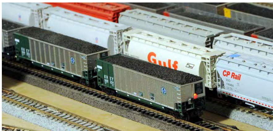
My BNSF coal train has resumed its journey to a distant power plant. The last car has just cleared the in-track magnet allowing the reed switch to relax and turn on the flashing red EOT device. Photo by Hugh Boyd
